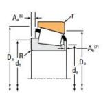
TS style is the most widely used tapered roller bearing.
